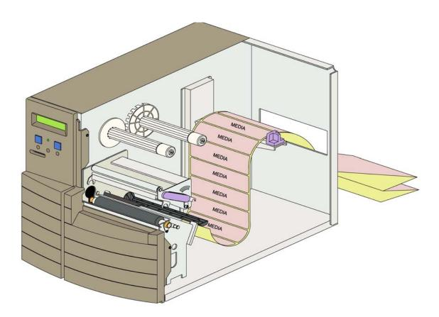
Figure 3-3b, Fan-fold Media Loading
